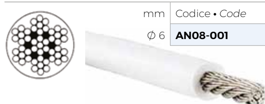
Cavo draglie in acciaio inox con rivestimento in PVC Flessibile 7x7 (49 fili) Ø 4 mm - Ø esterno con PVC mm 6 Stainless steel lifelines cable covered with PVC Flexible 7x7 (49 wires) Ø 4 mm - External Ø with PVC mm 6
